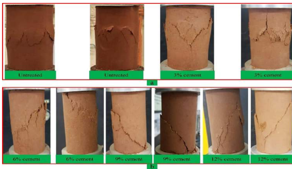
Figure 6. Failure plane for 28-day curing: (a) bulging shape (b) inclined shape.
