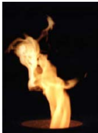
Figure 1.2 Precessing Vortex Core Flame [1]
