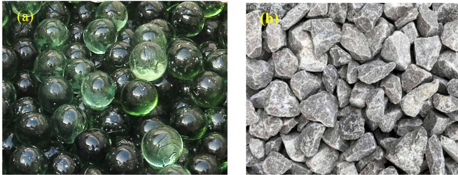
Fig. 1. Coarse aggregates used in this study
