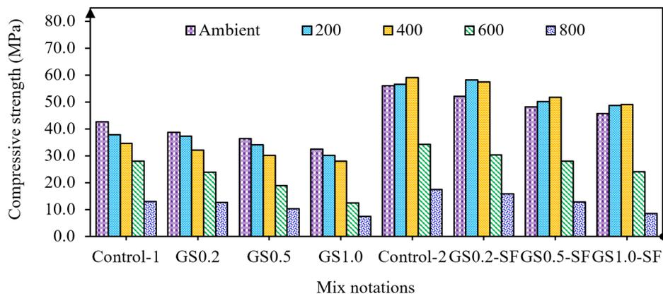
Fig. 5. Compressive strength of CRT concrete after exposure to high temperatures
