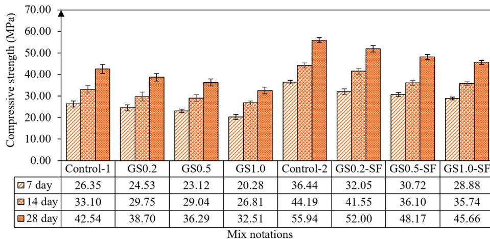
Fig. 4. Compressive strength of CRT concrete
