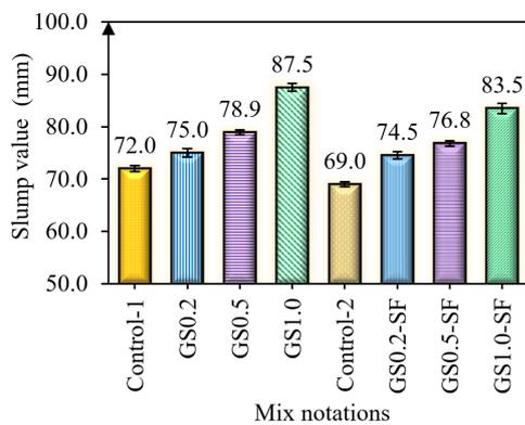
**Fig. 3.** Slump values of CRT concrete mixtures
