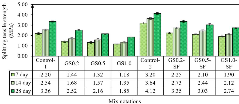
Fig. 6. Splitting tensile strength of CRT concrete
