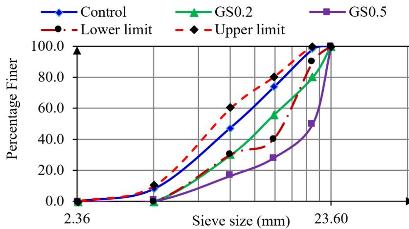
Fig. 2. Size distribution of coarse aggregates
