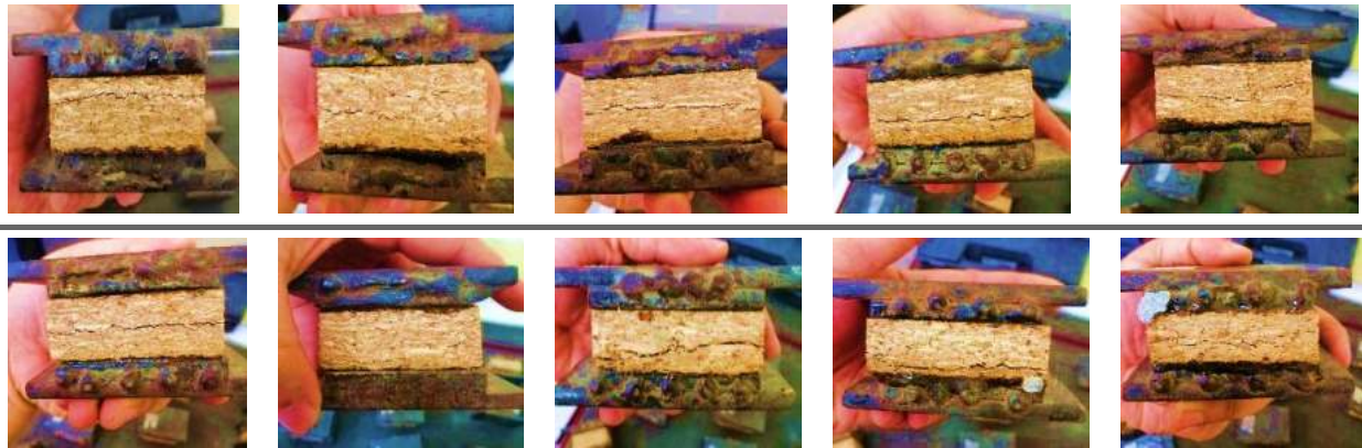
Figure 17. The crack of test pieces after failure for tensile strength.
