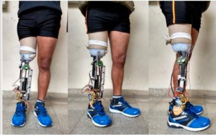
Figure 3: MR damper based prosthetic device [21]
