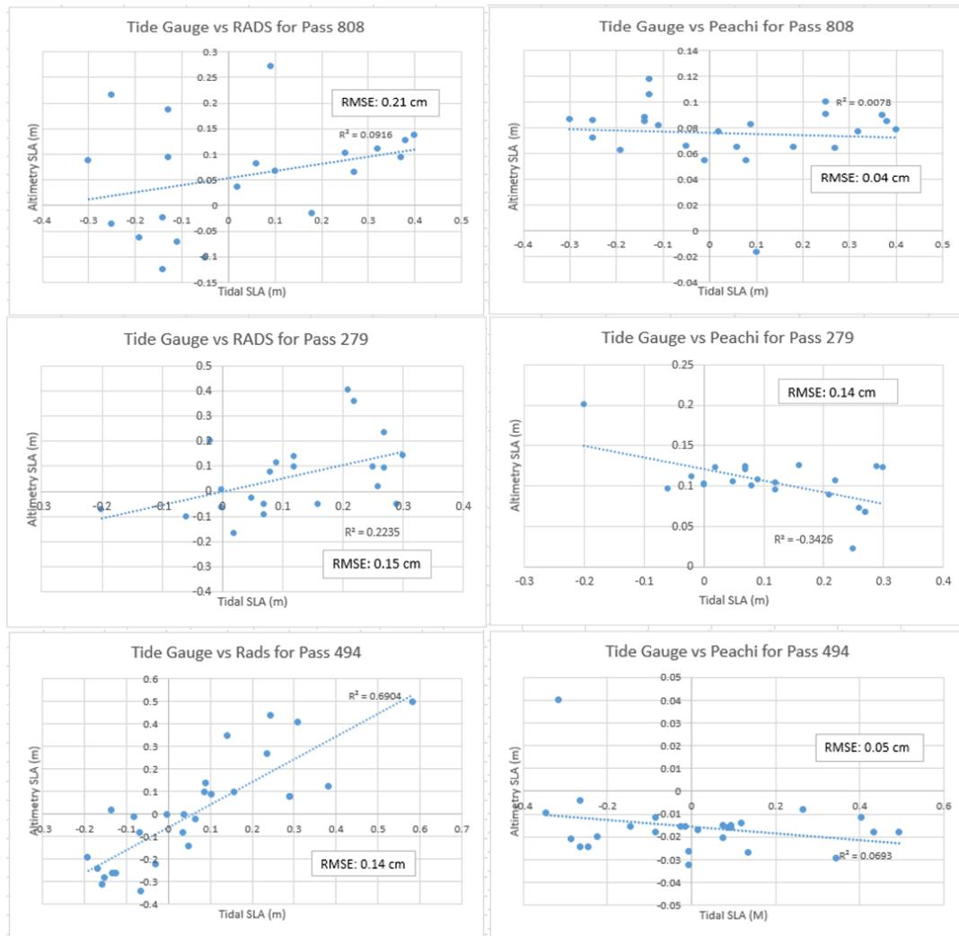
**Figure 8.** Correlation analysis, R<sup>2</sup> and RMSE comparison with sea level anomaly (SLA) from tide gauge versus RADS (left) and tide gauge versus PEACHI (right) at the selected tide gauge station.
