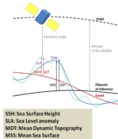
**Figure 2.** Difference between actual sea surface height (SSH) and the mean sea surface height (MSS) [11]
