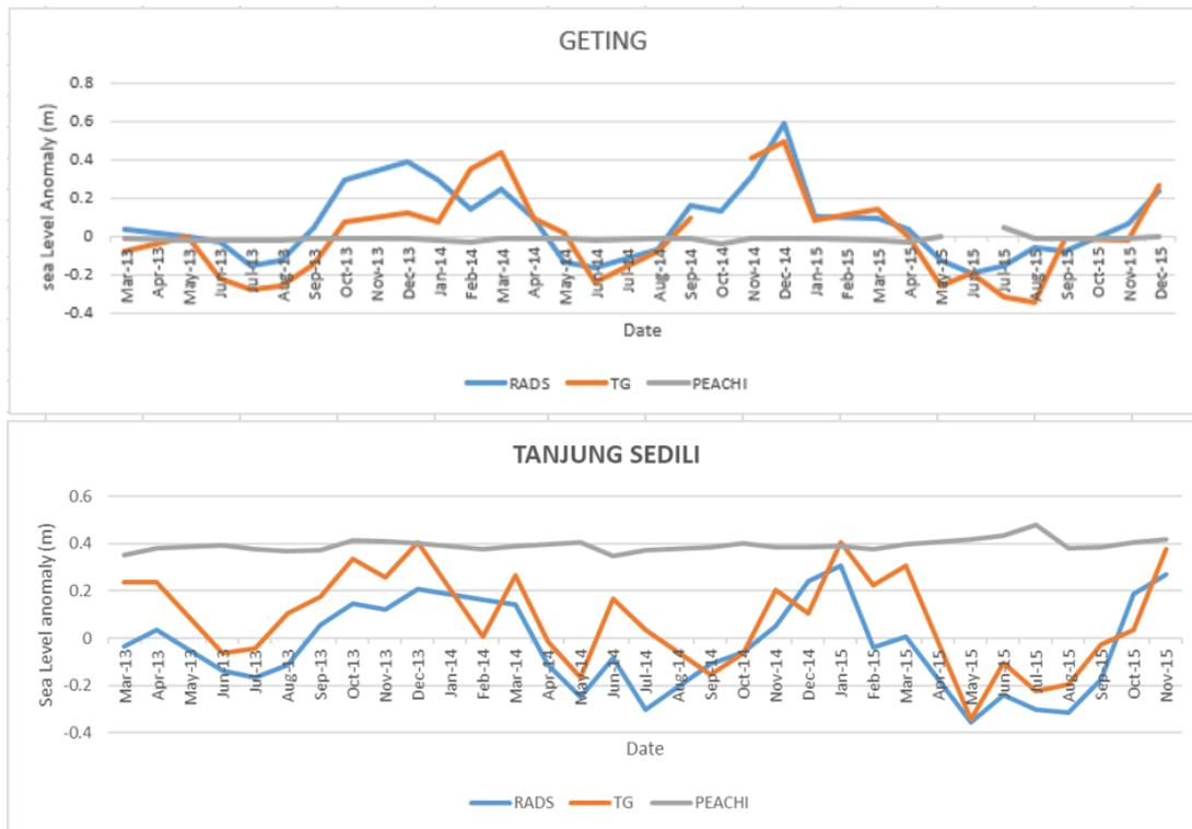
**Figure 7.** Comparison of time series trend from Tide Gauge (orange) with hourly sea level anomaly (SLA), RADS (blue) and PEACHI (grey) at the selected tide gauge station. Units are meter.
