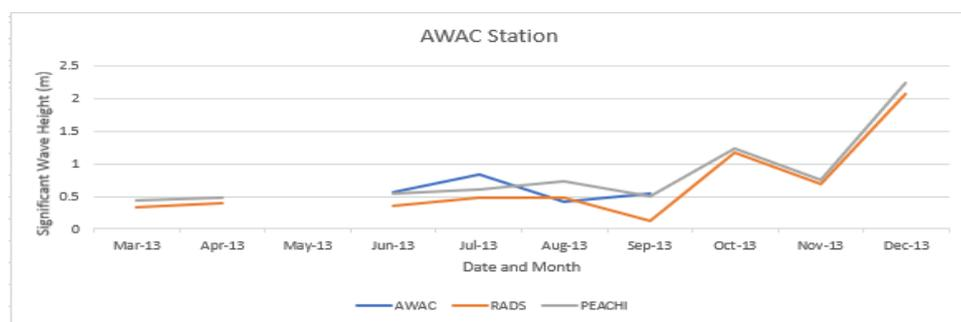
**Figure 9.** Comparison of time series trend from AWAC (orange) with hourly significant wave height (SWH), RADS (blue) and PEACHI (grey) at AWAC station (Peninsular Malaysia) using Pass 494 of altimeter track. Units are meter.
