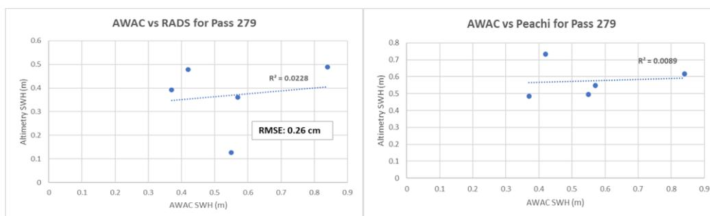
**Figure 10.** Correlation analysis,  $R^2$  and RMSE comparison with hourly significant wave height (SWH) from AWAC versus RADS (left) and tide AWAC versus PEACHI (right) at AWAC station (Peninsular Malaysia).
