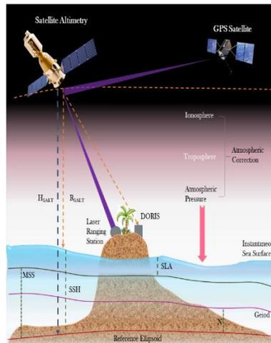
**Figure 1.** Principle measurements of satellite altimetry [9]
