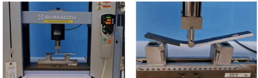
Figure 6. Experimental set up for the ENF specimen.
