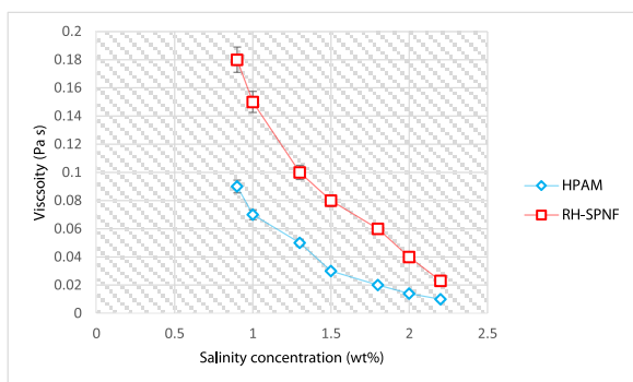
Fig. 8 – Effect of RH-SPNF on viscosity of HPAM solution as a function of salinity concentration.
