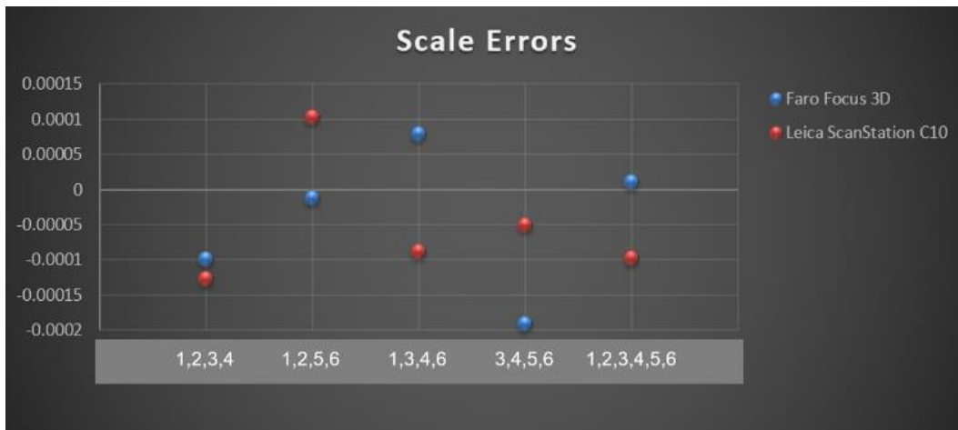
Fig. 9. Scale errors in multi sensors experiment for both phase and pulse-based scanners.
