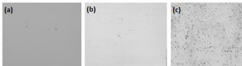
Figure 2. Image of acoustic cavitation bubbles under 20kHz ultrasound, (a) Non-degassed water, (b) Pure ethanol, (c) Ethanol-water mixture
