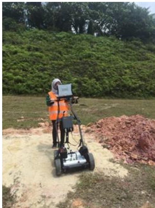
Figure 3. Observation on testbed of sand soil by using GPR RIS Hi-Mod.
