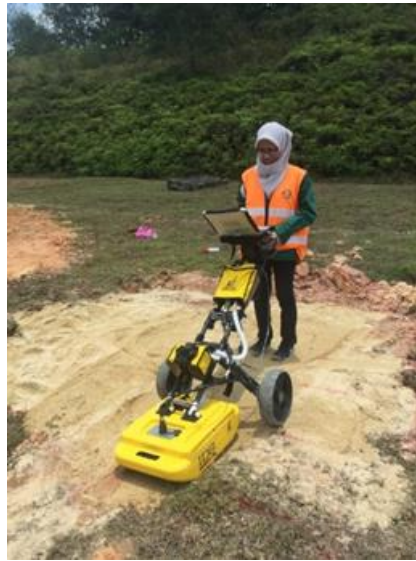
Figure 4. Observation on testbed of clay soil by using GPR IDS DuoDetector.
