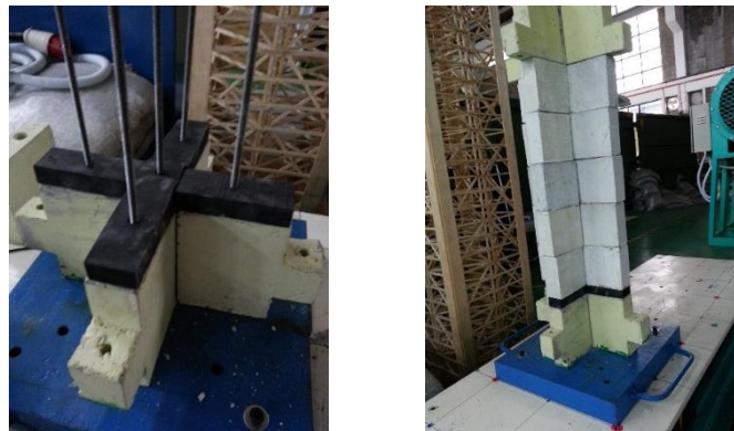
Figure 8. Setting up of hard rubber layer column on shaking table.
