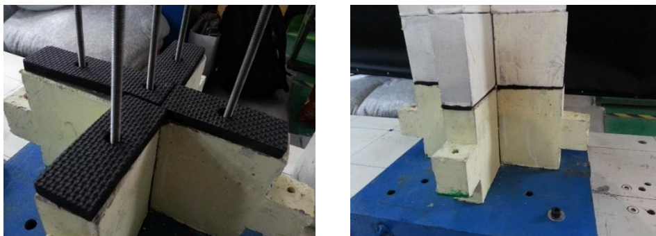
Figure 7. Setting up of soft rubber layer column on shaking table.
