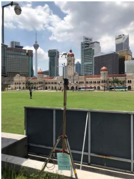
Fig. 3 Ultrasonic anemometer installed at D-M.
