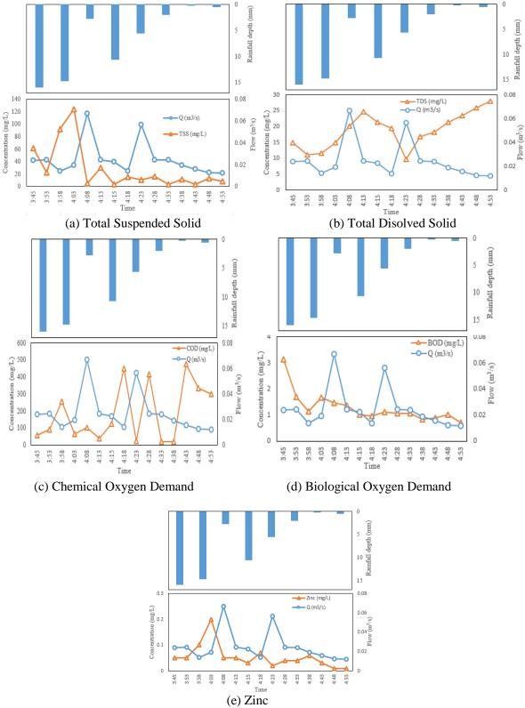
Figure 4. Hyetograph, hydrograph and pollutograph for the event.
