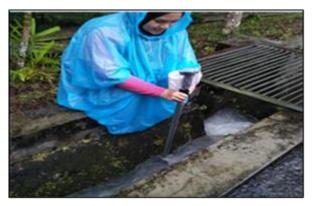
Figure 3. Measurement of runoff velocity
