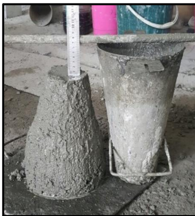
Figure 5. Slump cone test setup.
