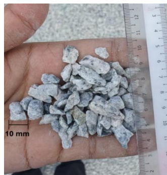
Figure 2. 10-mm course aggregate.
