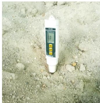
Figure 1. Few places within fine aggregate store were checked as to conform within the range using soil moisture meter.
