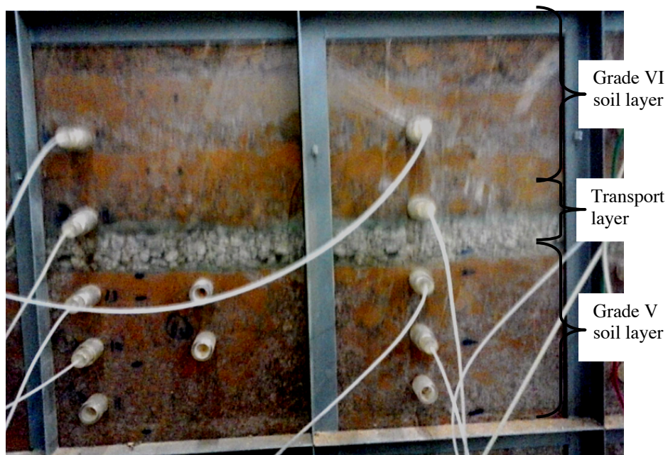
Figure 2. Section of prepared laboratory slope model with soils and transport layer before testing.
