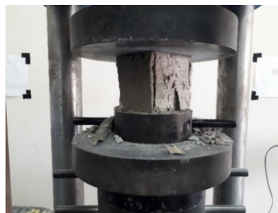
Figure 5. Sample for 40 MPa targeted strength was being tested.
