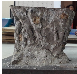
Figure 6. Sample for 40 MPa targeted strength after being tested.
