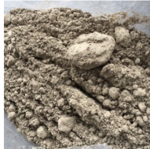
Figure 2. Class F fly ash used for geopolymer concrete mix.
