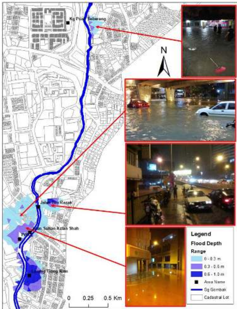
Figure 4. Flood extent from simulation results on 25 th December 2014 along Sungai Gombak.
