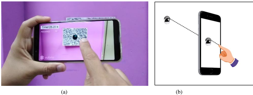
Figure 7. (a) common touch-based interaction (b) ray casting selection process.
