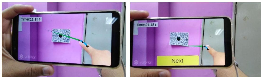
(a) User selecting 3D object using Ray-Casting technique (b) A button will be displayed after the object has been selected
