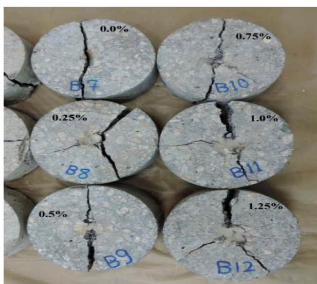
Figure 6. Failure modes of pumping method PAFRC specimens after impact load.
