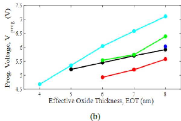
Fig. 2. Program Voltage,  $V_{prog}$  for each EOT of all VARIOT stack (a) Retention constraint >  $|-1.5V|$  (b) Read Disturb Constraint > 3.6V
