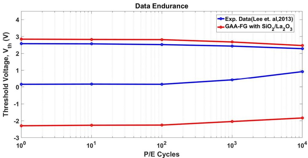
Fig. 5. Comparison of data endurance after  $10^4$  of P/E cycles between GAA-FG with  $\text{SiO}_2/\text{La}_2\text{O}_3$  and single stack,  $\text{SiO}_2$ . Wider threshold shift can be observed for  $\text{SiO}_2/\text{La}_2\text{O}_3$  stack resulting to a better endurance (16% data loss) compared to the single stack (46% data loss).
