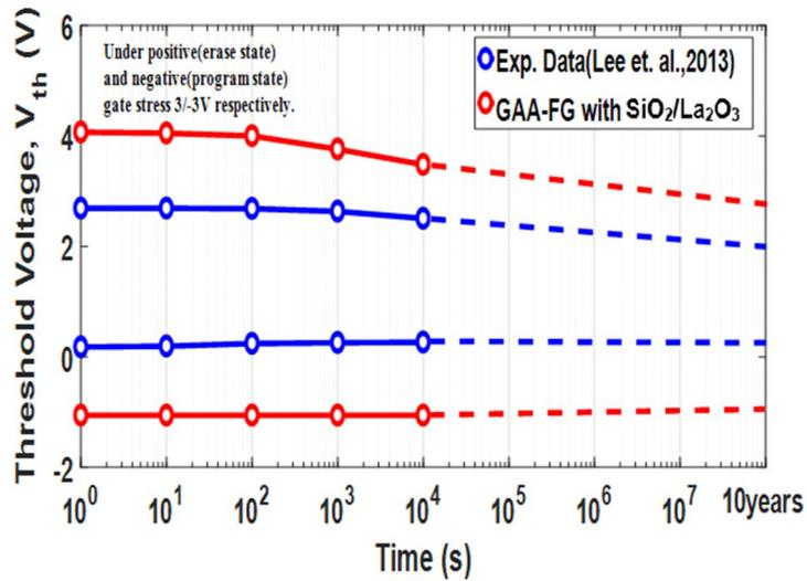
Fig. 4. 10 years approximation of data retention under positive (erase state) and negative(program state) gate stress 3/-3V. For a given P/E operational time, engineered tunnel stack shows steeper slope and wider memory window compared to experimental data.
