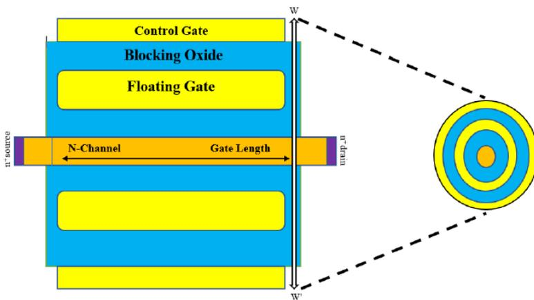
Fig. 1. Cross-section of 3-D GAA-FG with SiO<sub>2</sub>/La<sub>2</sub>O<sub>3</sub> tunnel stack. The physical thickness for tunnel stack is 22nm where SiO<sub>2</sub> layer is 1nm.
