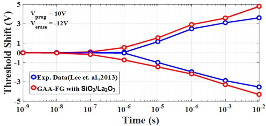
Fig. 3. Threshold voltage shift of GAA-FG for 10/-12V operational voltage. Engineered tunnel stack reduced the P/E operational speed for a fixed P/E voltage and time. As shown in the figure, the FG is charged earlier at  $\sim 10^{-6}$  s for  $\text{SiO}_2/\text{La}_2\text{O}_3$  stack and led a wider memory window than experimental data
