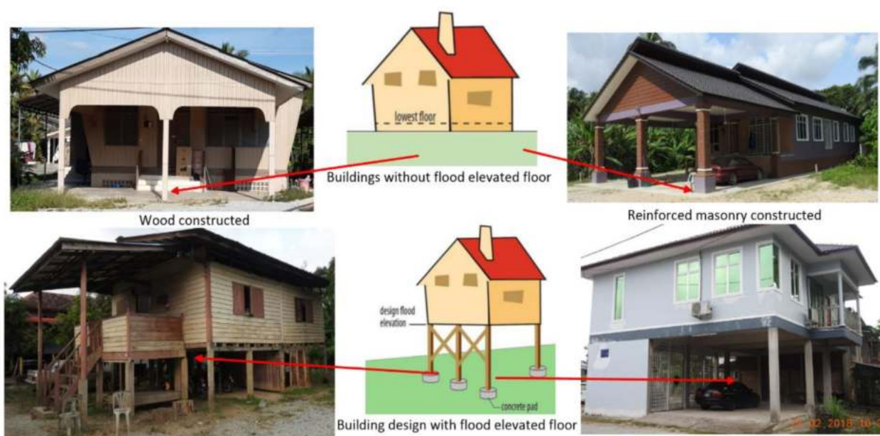
Figure 13. An illustration of elevated and non-elevated buildings.
