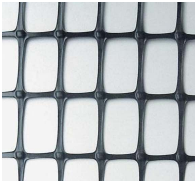
Fig 5. Polymeric extruded biaxial geogrid type BX1500 [62].
