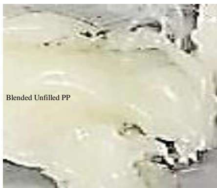
Figure 1. Polypropylene sample prepared by means of Brabender melt mixer
