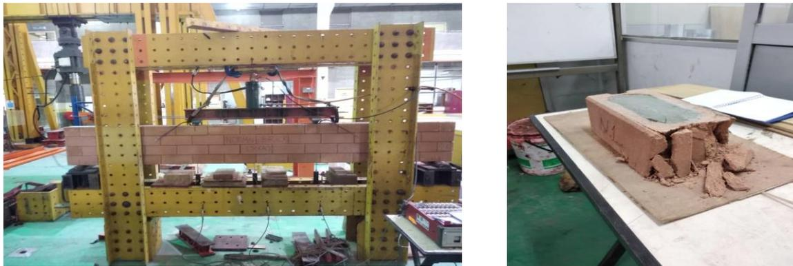
**Figure 5.** Specimen properties and testing and failure mode due to compression.
