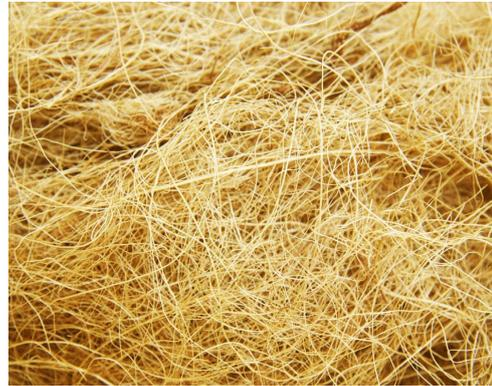
**Figure 3.** Palm Oil Fibre.
