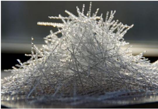
**Figure 2.** Synthetic Polypropylene Fibre (SPF).
