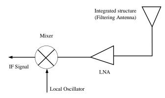
Figure 1.2 Block diagram of RF front end with integrated structure
