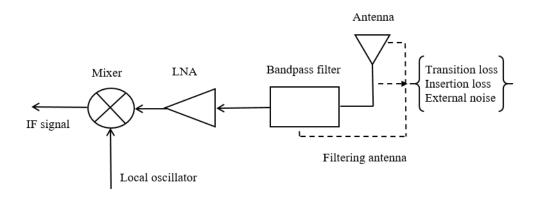
Figure 1.1 Block diagram of RF front end receiver
