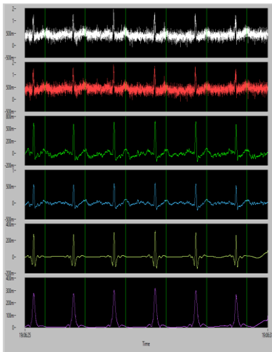
Figure 4. (a) Raw ECG signal acquired by one of the healthy subjects; (b) After applying the notch filter (47 to 53 Hz); (c) IIR Band Pass filtered (0.05 to 20 Hz); (d) FIR high pass filter using Kaiser window (order of 56 and cut-off frequency of 3.5 Hz); (e) Denoised signal; (f) R-peak detected by the multiresolution wavelet transform.
