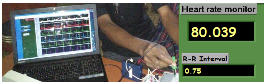
Figure 5 (a). ECG acquisition and heart rate monitoring device
