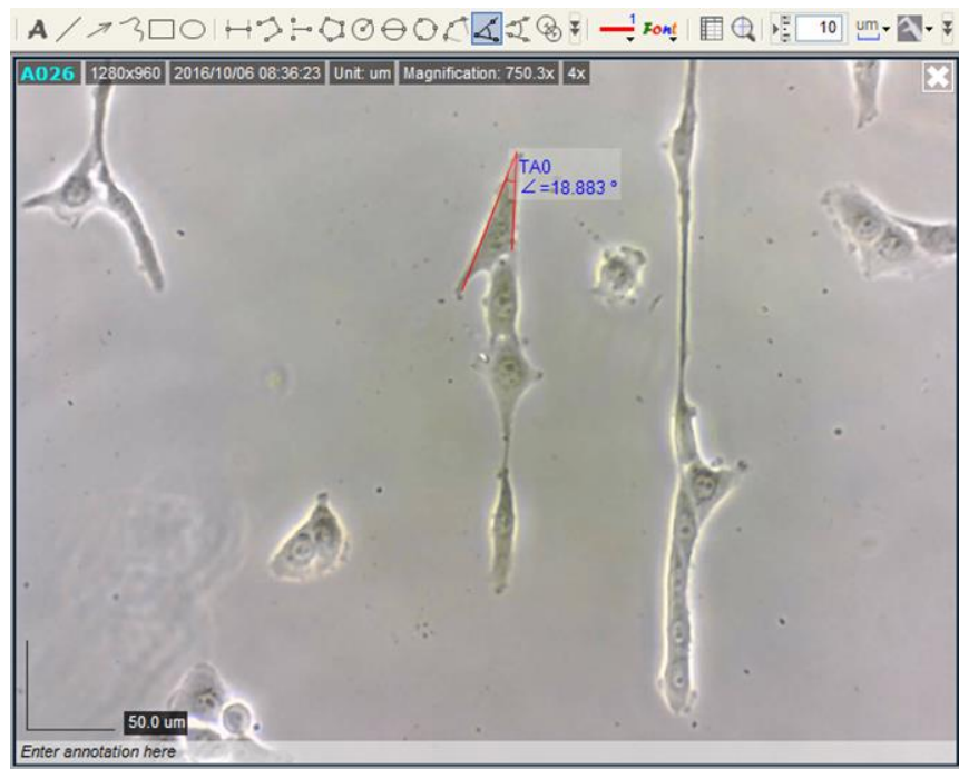
Figure 2. An example of angle measurement with DinoCapture2.0 software.
