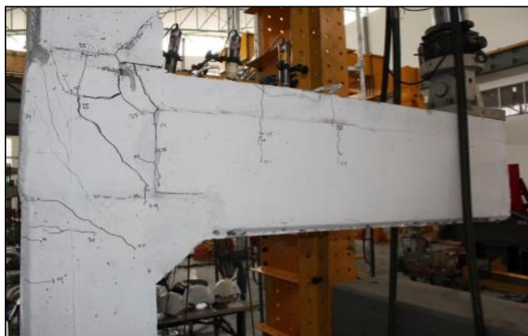
Figure 9. Failure mode of precast beam [2].
