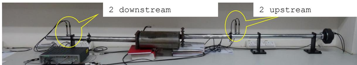
**Figure 2.** Complex muffler setup.
