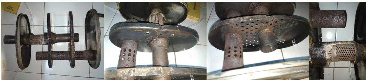
**Figure 3.** Complex muffler internal geometry.
