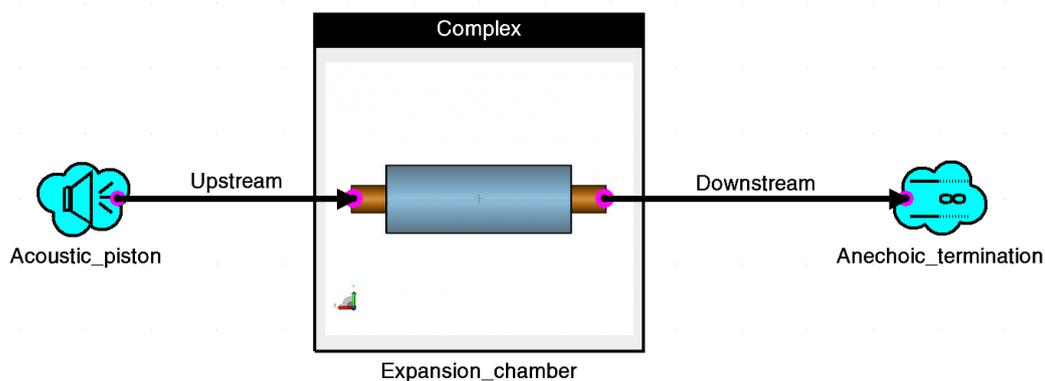
**Figure 4.** Big expansion chamber 1D simulation setup.
