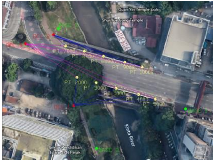
Figure 7. Line of Sight from Occupy Station to Monitoring Points
