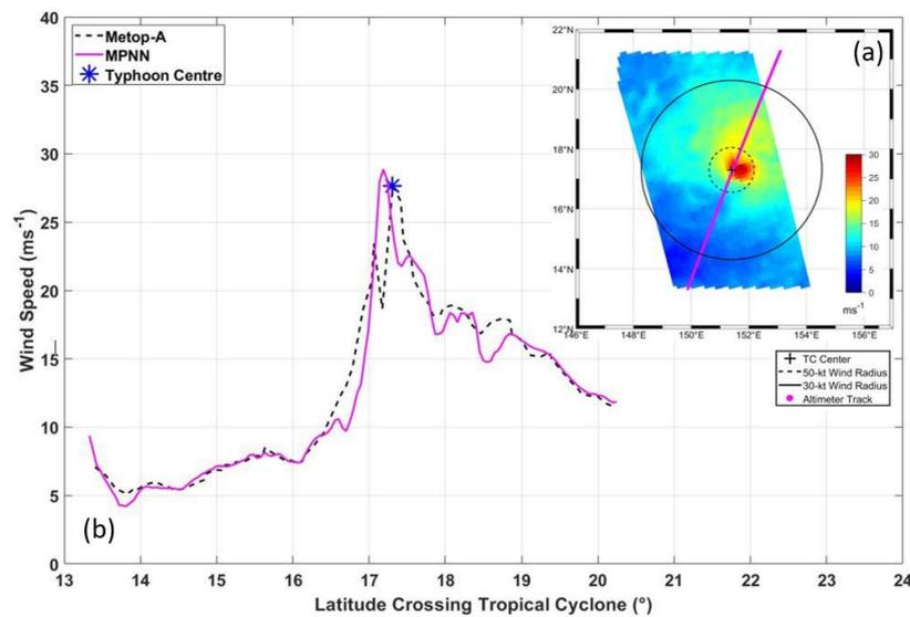
**Figure 5.** Typhoon Jebi wind radius from the JMA best track report on 29 August 2018 at 12:00 with Metop-A wind speed map and Jason-2 crossing track are shown in (a). The profile of wind speed derived from MPNN and Metop-A match-up is shown in (b) represents the tropical cyclone wind structure.
