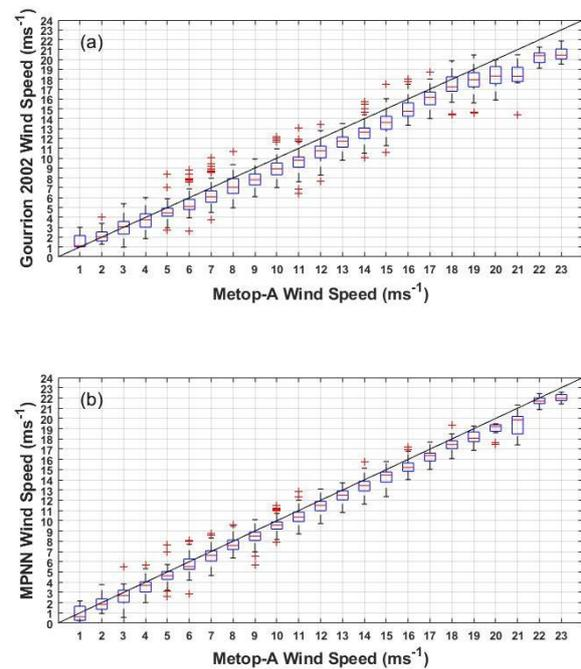
**Figure 4.** Box-whisker plot of the Gourrion 2002 (a) and MPNN (b) estimated wind speed against Metop-A.
