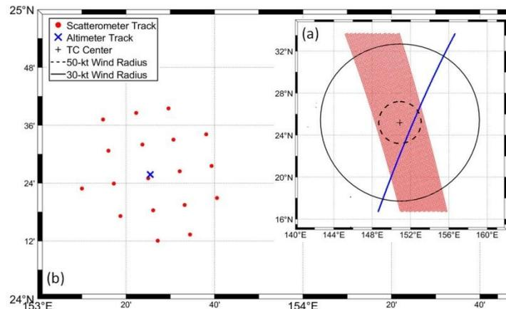
**Figure 1.** Data match-up between Jason-2 and Metop-A observation as both satellites crossing tropical cyclone event in (a). A closer look of  $1 \times 1^\circ$  grid into a single Jason-2 point in blue cross with multiple Metop-A points at centre of pixels in red dots depicted in (b).
