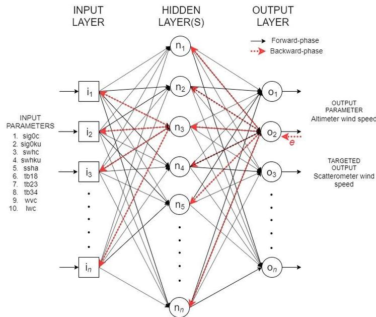
**Figure 2.** The processing architecture of the neural network of forward- and backward-phase. The  $i_1$  to  $i_n$  is the number of match-up data used in training (in this case, 60% of the samples) which resulted in the  $o_1$  to  $o_n$  output of the wind speed estimate. The  $n_1$  to  $n_n$  is the number of processing neurons assigned to the corresponding hidden layers.
