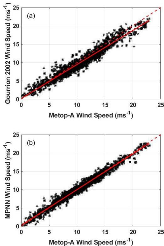
**Figure 3.** The scatter plot of the wind speed estimates using the raw Jason-2 as a function of Gourrion 2002 model (a) and the MPNN (b). Black asterisk shows the match-up points, red solid-line is the estimated linear fitting, and red dashed-line is the best fit.
