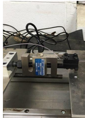
Figure 2. Fabricated tensile test for fiber optic. Figure 3. Load cell to obtain tensile force data.
