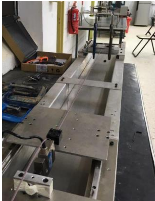
Figure 2. Fabricated tensile test for fiber optic. Figure 3. Load cell to obtain tensile force data.
