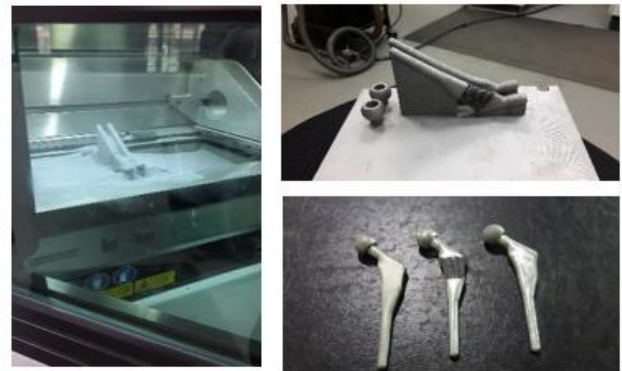
Fig. 3. Fabrication of hip implant using direct laser metal sintering.
