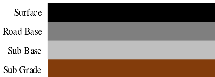
Figure 1. Structure in flexible pavement.
