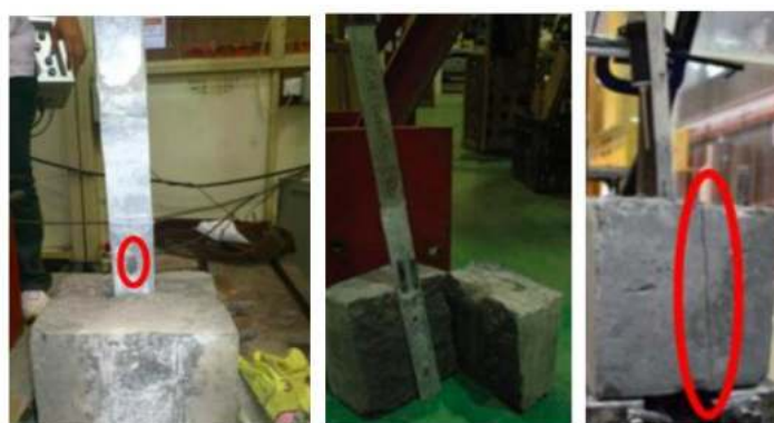
Figure 7. Failure modes of pull-out test of FC with cold-formed steel strips [152–154]. Reprinted with permission from [152–154].
