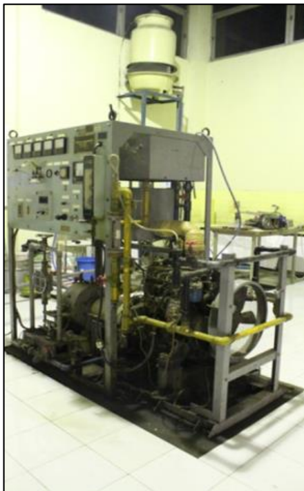
Diesel Engine Test Bed (2018)
