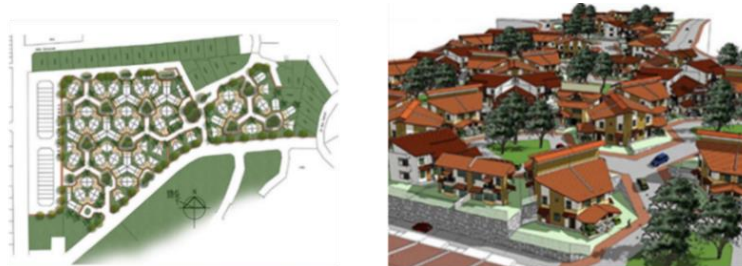
Figure 4. The ‘honeycomb’ layout concept applied in NongChik, Johor Bahru Source: An original figure from Ghazali (2007) in Affordable Low and High-Rise Honeycomb Housing [21]
