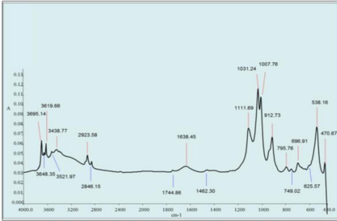
**Figure 3.** FTIR spectra for natural laterite clay soil
