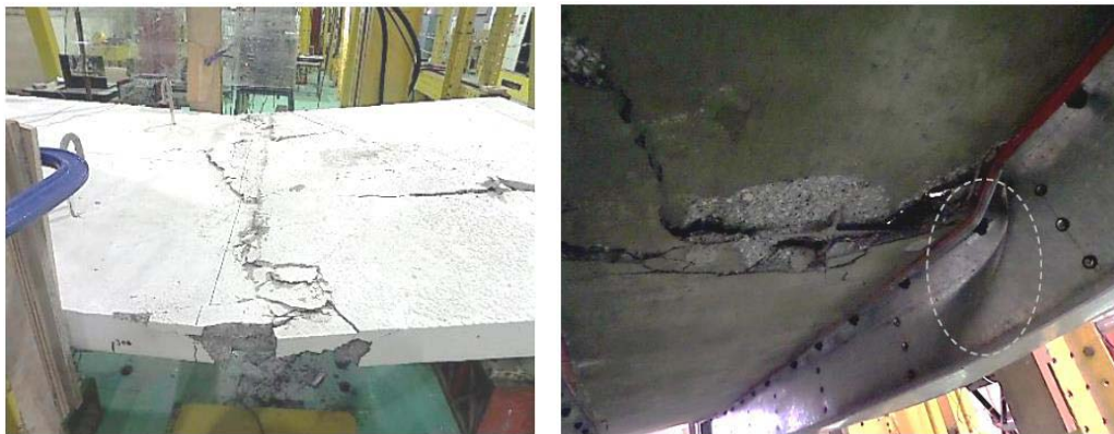
(a) Concrete crushing
