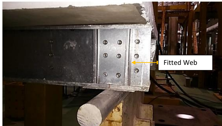
Figure 2. Fitted web at support position.
