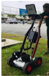
Figure 6. RIS HI-MOD GPR with dual frequencies 400 MHz and 900 MHz antenna systems.
