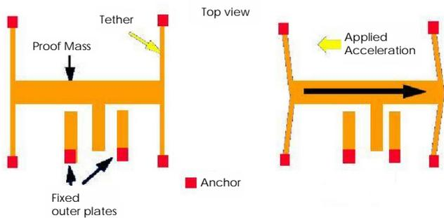
Fig. 7. Accelerometer assembly structure [61].
