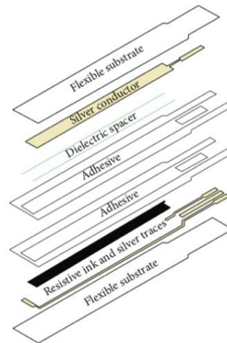
**Fig. 5.** MEMS flexible force sensor details [c].
