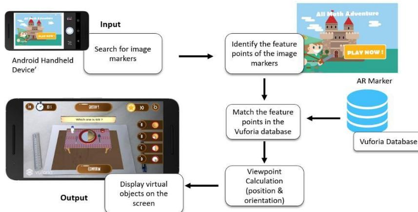
**Figure 5.** Feature-based tracking workflow using Android handheld camera with Vuforia SDK.
