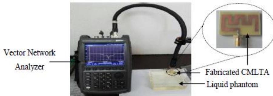
Figure 5. Measurement setup: CMLTA in developed phantom
