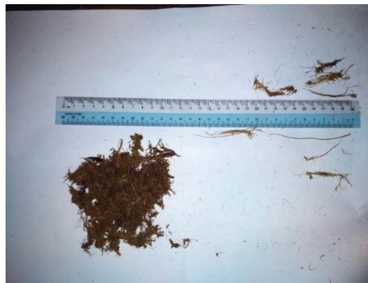
Figure 1.2 Conditions of the PPMF from the mechanical screw press that will be conveyed into the hexane extraction plant.
