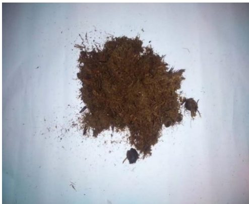
Figure 1.2 Conditions of the PPMF from the mechanical screw press that will be conveyed into the hexane extraction plant.
