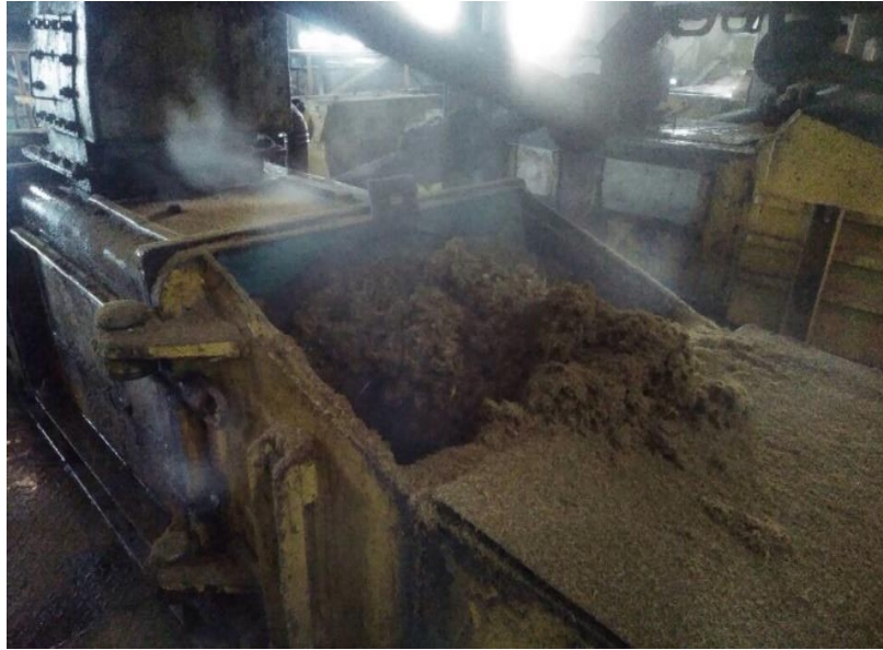
Figure 1.1 Palm mesocarp fiber being expelled out from the mechanical screw press after pressing at the palm oil mill.
