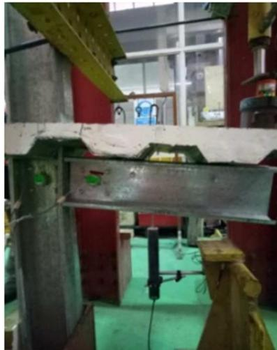
Figure 7. Condition of Specimen 1 at ultimate failure
