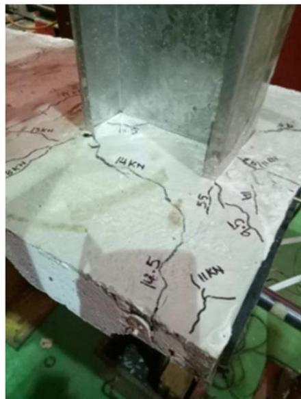
Figure 9. Cracking near to the column in tension zone
