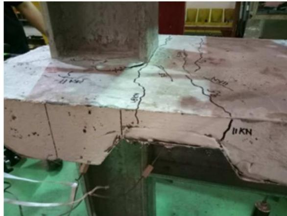
Figure 8. Transverse cracks on concrete slab
