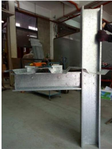
Figure 4. Bolt arrangement and profiled steel decking
