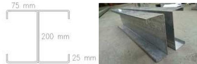
Figure 2. Cold-formed lipped C-channel sections
