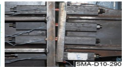
Figure 10. Detailed connection deformation ([37])
