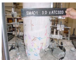
Figure 16. Specimen SMAC-1 after Run 11 [46]
