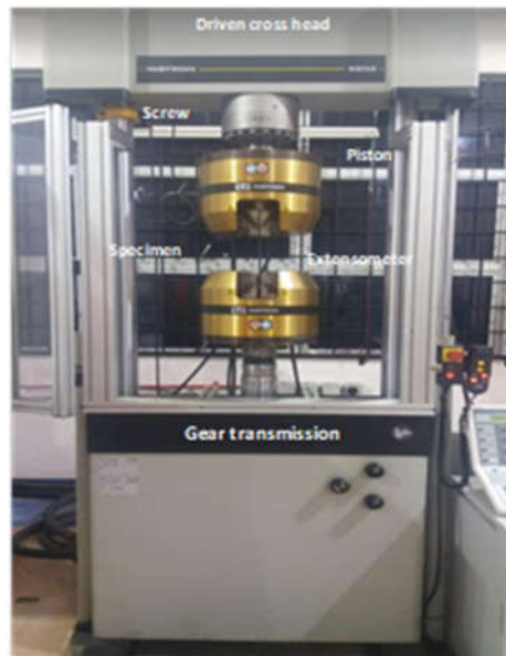
Figure 3. Schematics Showing of a Hydraulic Testing Machine for Instron Testing apparatus model 600 DX used for experiment.
