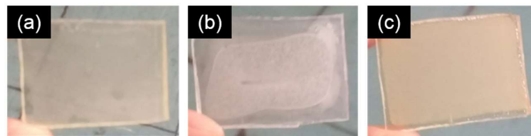
Figure 3. Photographs of coated PC sheets by using drop-casting method with TiO_2 suspensions prepared by (a) method 1, (b) method 2 and (c) method 3.
